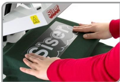
Align the transfer material on the garment to be printed and cover with a cover sheet.
